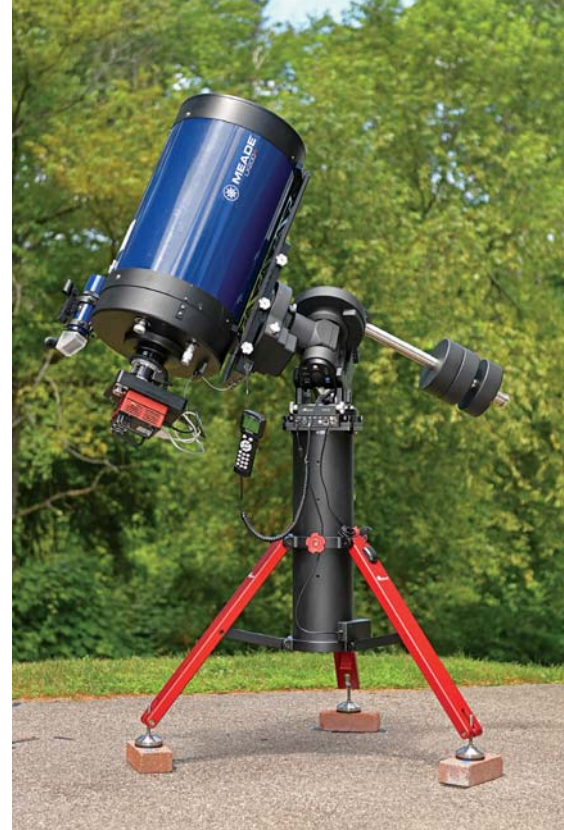
▲ As described in the text, the author tested the CEM120 for visual observing and CCD imaging with a Meade 14-inch Schmidt-Cassegrain optical tube assembly fitted with accessories that brought the total load weight to about 85 pounds.
